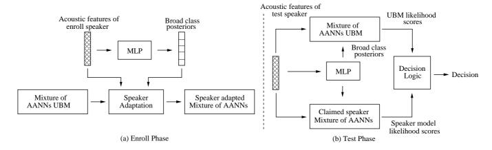
Figure 2: Enrollment and testing using a mixture of AANNs
