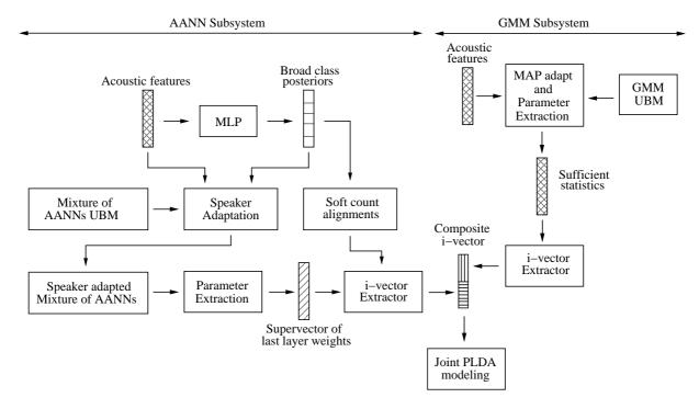
Figure 3: Creating AANN and GMM based i-vectors for joint PLDA modeling
